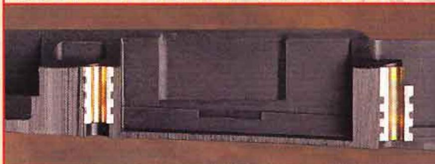
Pillar Bedding is used to enhance accuracy by providing maximum stability for the action. "Dual Pillar" bedding is accomplished by permanently embedding two steel pillars in the stock. Front and rear action screws are inserted through the two pillar sleeves into the receiver to provide steel-to-steel contact points.
