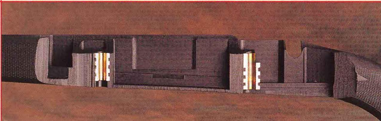
Pillar Bedding is used to enhance accuracy by providing maximum stability for the action. "Dual Pillar" bedding is accomplished by permanently embedding two steel pillars in the stock. Front and rear action screws are inserted through the two pillar sleeves into the receiver to provide steel-to-steel contact points.
